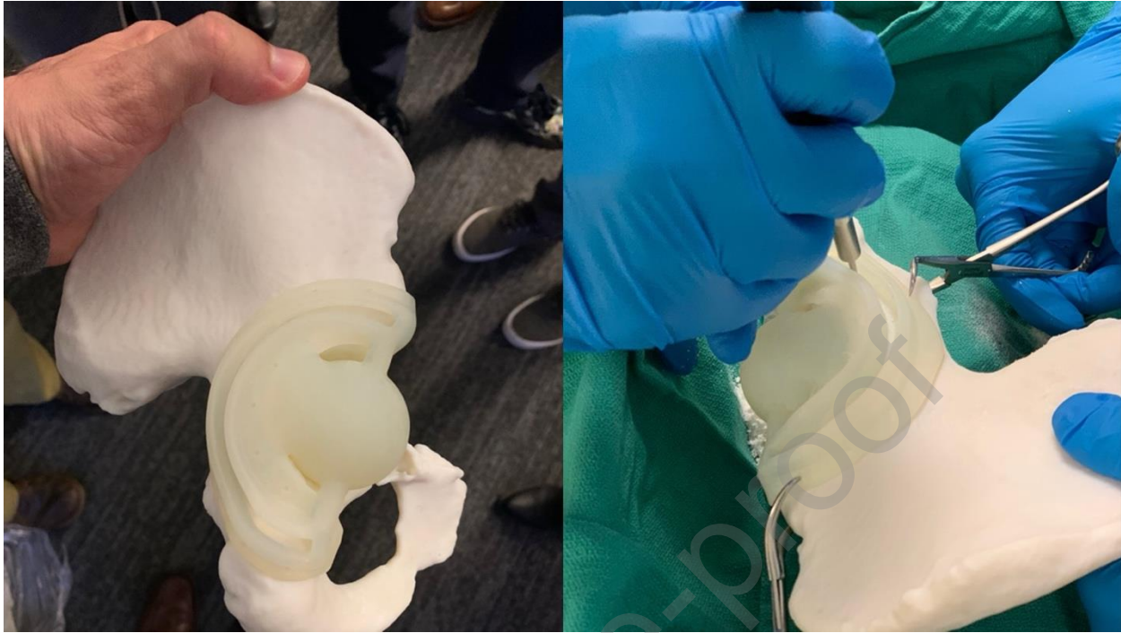
Figure 3. Use of 3D-printed PSIs allow operative rehearsal and fast, low-cost iterative improvements to the design through surgeon feedback and testing
